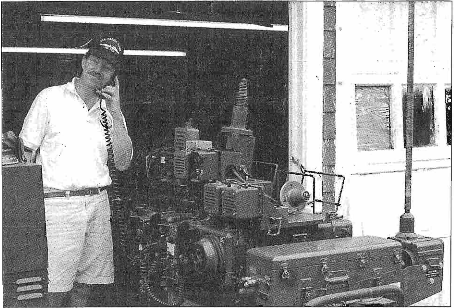
Brown, W1NZR, on VFD with a MRC-108/GRC-153 vehicle mounted HF, VHF, UHF radio communications set.
