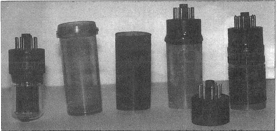
Fig.1. Low cost plug-in coil forms can be made from pill bottles and tube bases.
