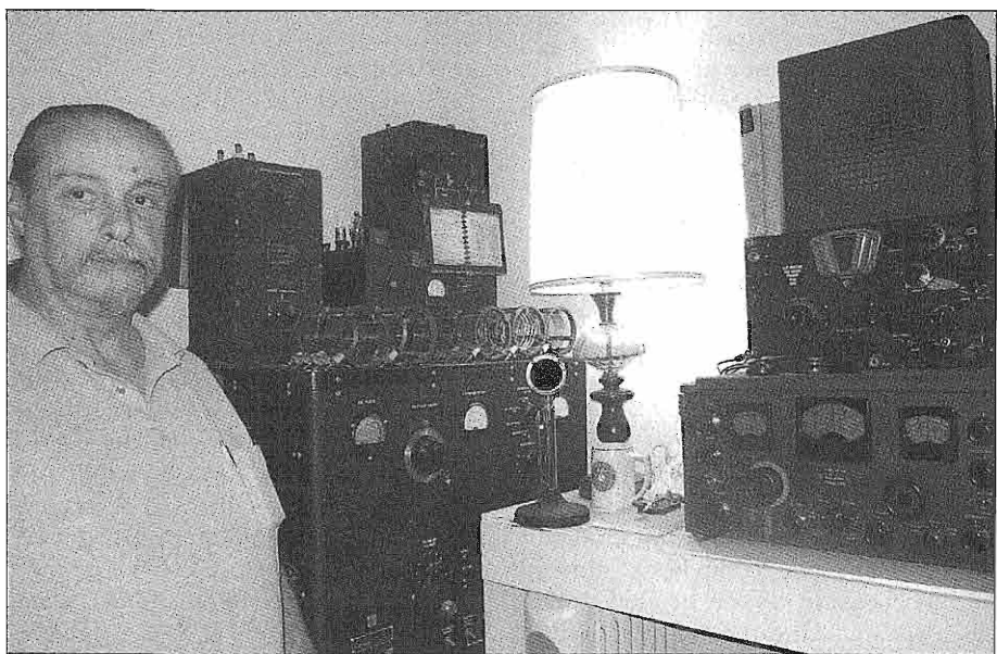
John Hruza, KBØOKU, at his main military station. A Detrola BC-614-E speech amp drives the Bogen BC-610-F. The BC-306-A antenna tuner awaits a BC-639 replacement. Freq meter is a Hallicrafters BC-221-HA. Receivers are BC-312 and AN/GRR-2 (Hallicrafters SX-28).
