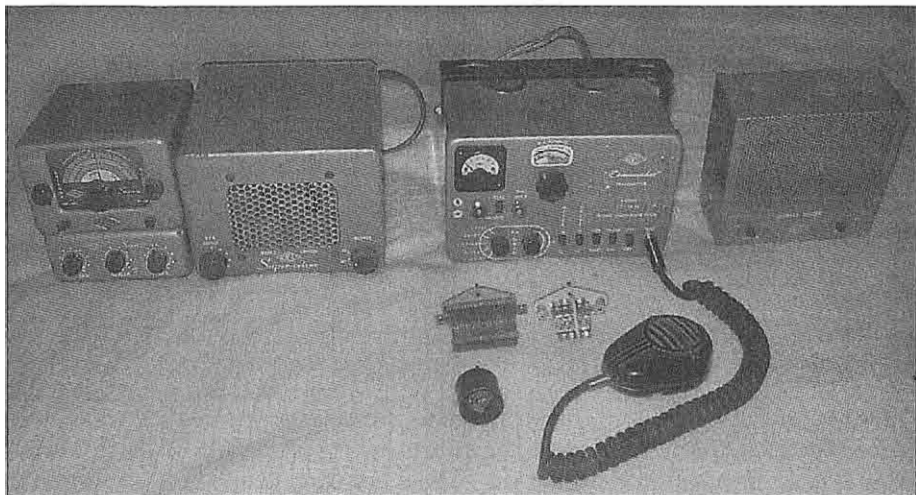
Figure 2: Left to right is shown the Gonset Super-ceiver with a 262 kc IF and an attached Super 6 converter. Center stage is the Gonset Commander, 1.7 to 54 mc, 35 to 50 watt AM transmitter with its original set of 4 plug-in coils. The Commander measures 8.5" X 5 3/8" X 7 1/8" deep. On the right side is the classic Gonset Signal Slicer that used a 455 kc IF.
