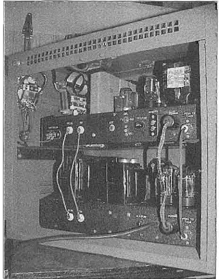
The Champ's RF deck (top) and power supply (lower).
