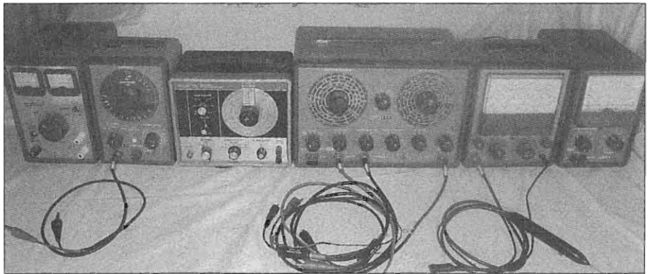
Figure 3 shows a typical third-generation test bench. Now, FM alignments are necessary, and made possible by the Type 369 shown fourth from the left. The 369 was an excellent piece that is still used by many technicians.
