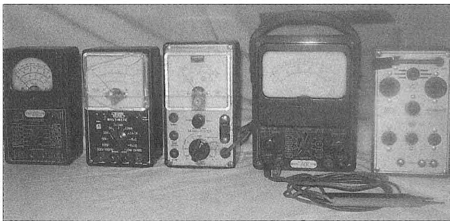
Figure 1, First and second generation EICO VOM equipment, with the type 612 filament checker shown on the far right.
