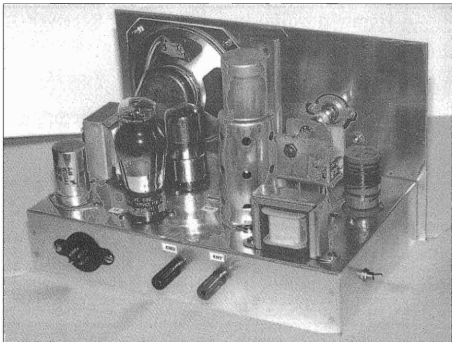
Figure 2 presents the rear view of the homebrew shortwave receiver. The locations of major components are clearly indicated, from the type 42 output on the left, to the plug-in coil and tuning condenser on the right.
