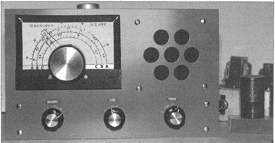
Figure 1 is the front-panel view of the classic W2HBE shortwave receiver. To the right are finished coil sets, pictured just ahead of the power supply described in Electric Radio #164 , January 2003.
