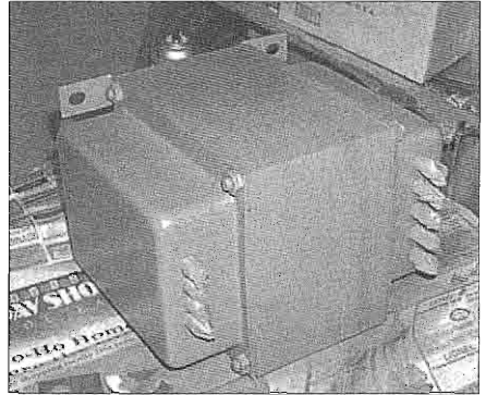
The big power transformer has been cleaned and painted as described in the text.
