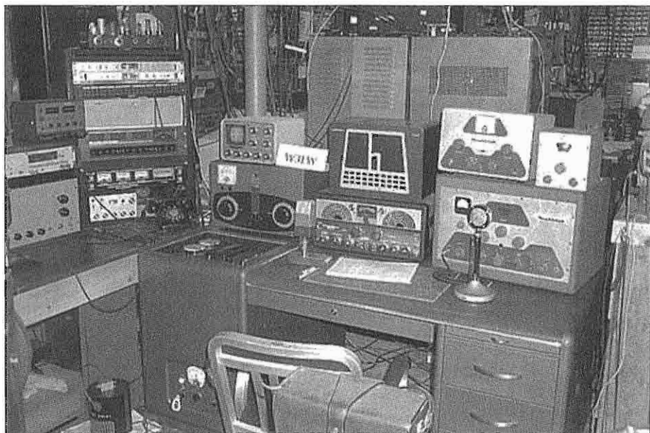
This is the main AM operating position at W3LW with the restored Johnson Desk KW and Matchbox tuned up and ready to go on 40 meters. The Hallicrafters SX-100 makes a perfect match to this classic station.
