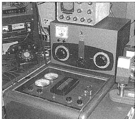
The Johnson Desk Kilowatt has been reassembled and is ready for 7290 kc.
