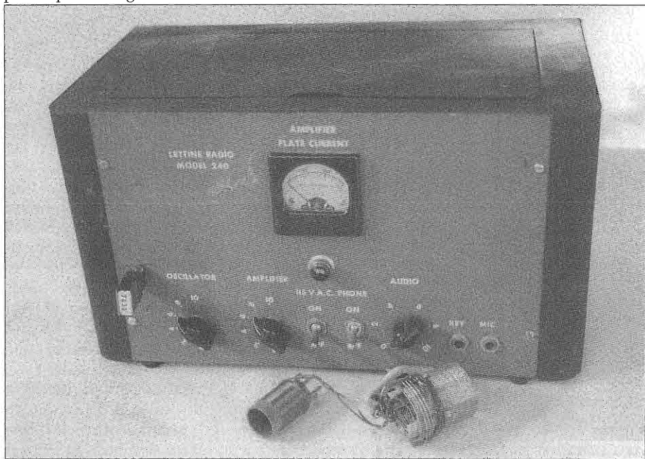
Figure 1: The 80-meter oscillator and final plate coils with their neutralizing links attached sitting in front of the Lettine 240.
