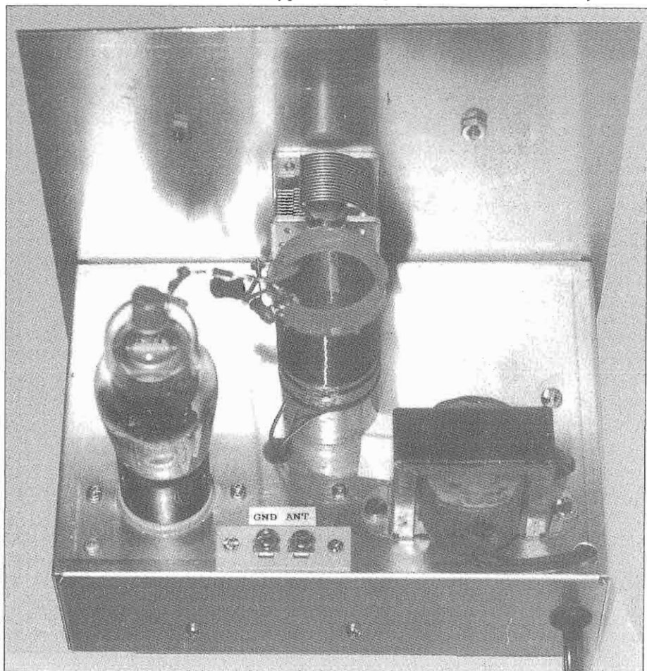
Figure 2: A view behind the front panel shows the homebrew coil form in the Novadyne.
