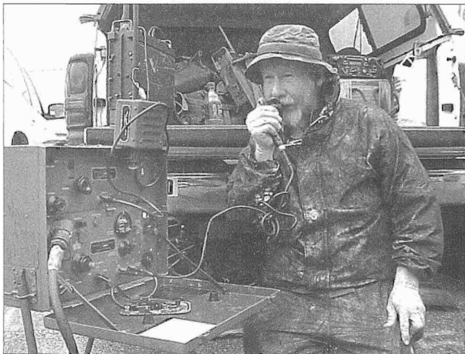
Here is the author operating his authentic BC-654 in the rain. The installation includes a T-17 hand mic and LS-8 loudspeaker.
