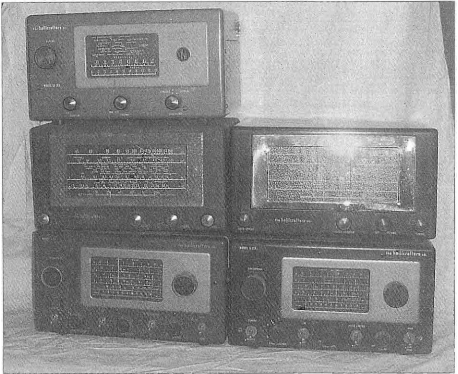
Figure 4: Here are some more familiar Hallicrafters monitor receivers. The top row holds an S-104 30-50 mc receiver, and the middle row has an S-94 30-50 mc receiver, and an S-95 152-173 mc receiver. In the bottom row from the left is the 2-meter S-102 and the 6-meter S-106.
