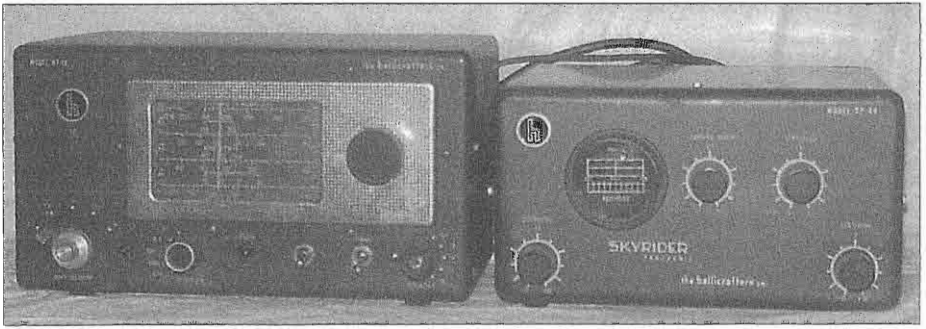
Figure 6: On the left is an HT-18 VFO/exciter. These were produced from 1947 to 1949 and covered 80 to 10 meters. They produced CW and NBFM emissions from a 6BA6 crystal or VFO oscillator, and a 6L6 multiplier and PA. They could generate about 5 watts of carrier. Two other 6BA6's served as the speech amplifier and FM reactance modulator. It had an internal regulated power supply, and a link-coupled output network. On the right is the SP-44 Skyrider Panadaptor. Note the slightly different case, originally produced by Panoramic Radio.
