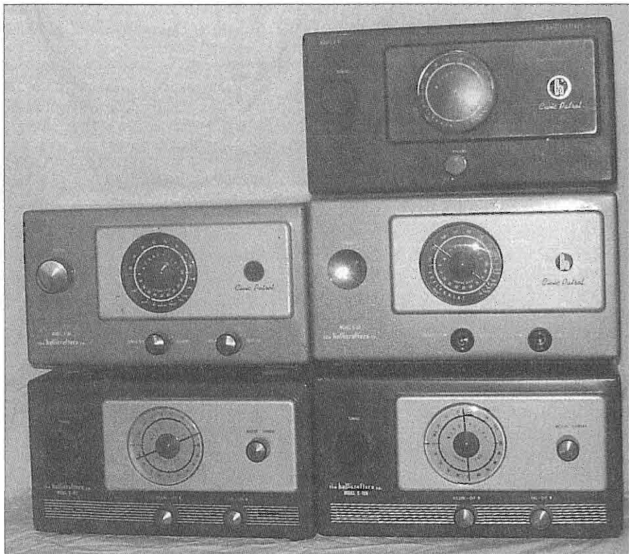
Figure 3: Here are several monitor receivers based on the S-38 cabinet design. The top row has the S-81, 152-173 mc "Civic Patrol" model. The middle row shows the S-94 30-50 mc and S-95 152-173 mc examples. In the bottom row an S-102 2-meter receiver is on the left, and an S-106 6-meter version is on the right.
