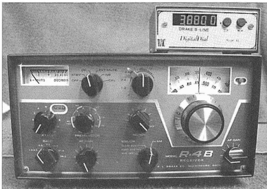
The RAC Digital Dial is small enough to sit on top of my Drake R-4B
