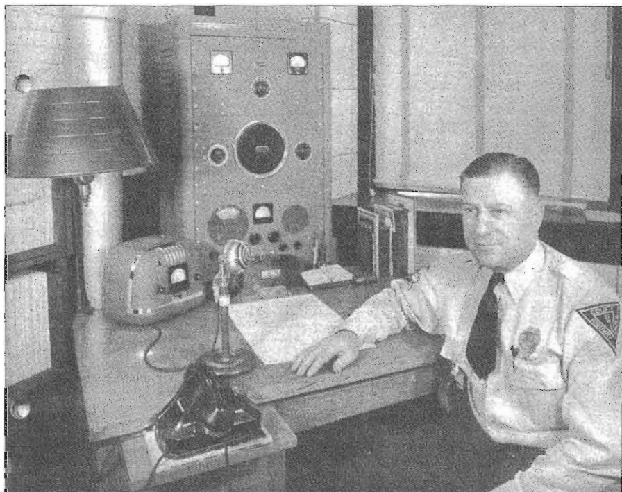
Taken about 1939, Captain Olson of the Wisconsin Highway Police is proud of his new Motorola T19-32H 31-Megacycle radio system. Vintage Motorola remotes for the T19 system are in the picture, as is a rack-mounted S-20R.
