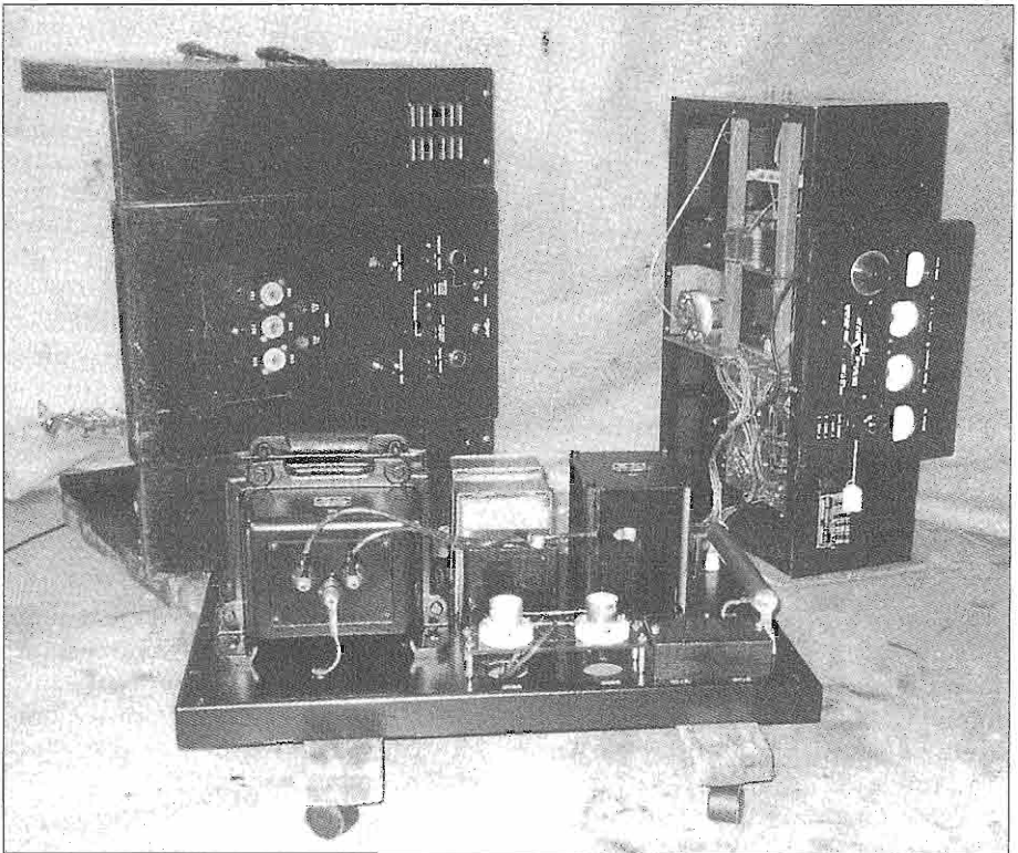
The BC-610E is broken down into the power supply deck (foreground), RF deck (right background), and modulator deck (left background).
