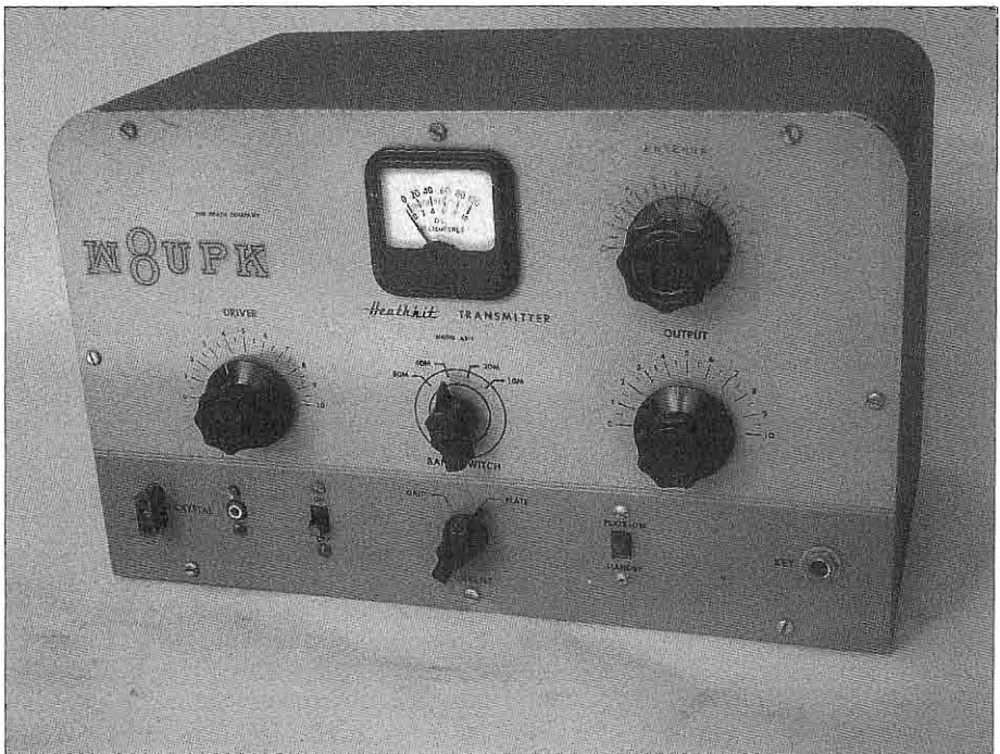
The Real McCoy Heathkit AT-1. The antenna loading knob controls a capacitor in series with the output link.
