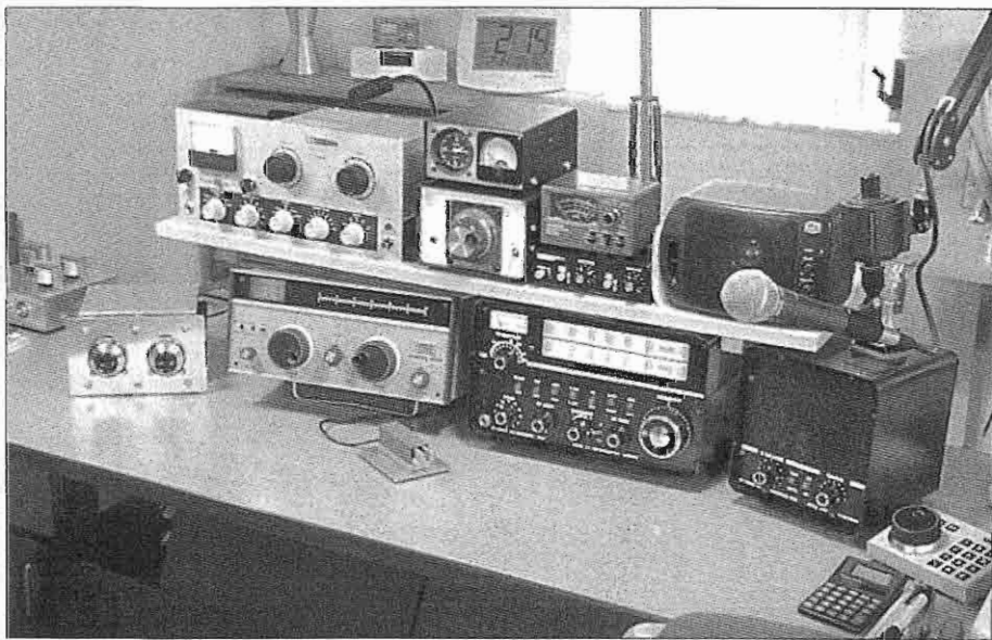
This is my present station with a Drake 2-B receiver, 2-BQ speaker/Q-multiplier, and a Heathkit DX-60 transmitter on the top shelf.
