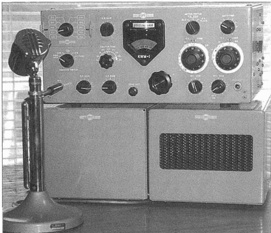
The KWM-1 at WA9MZU is pictured above with the 516F-1 115 VAC power supply and the matching 312B-1 speaker cabinet. A traditional Astatic 10-D microphone completes this late 1950s SSB station.
