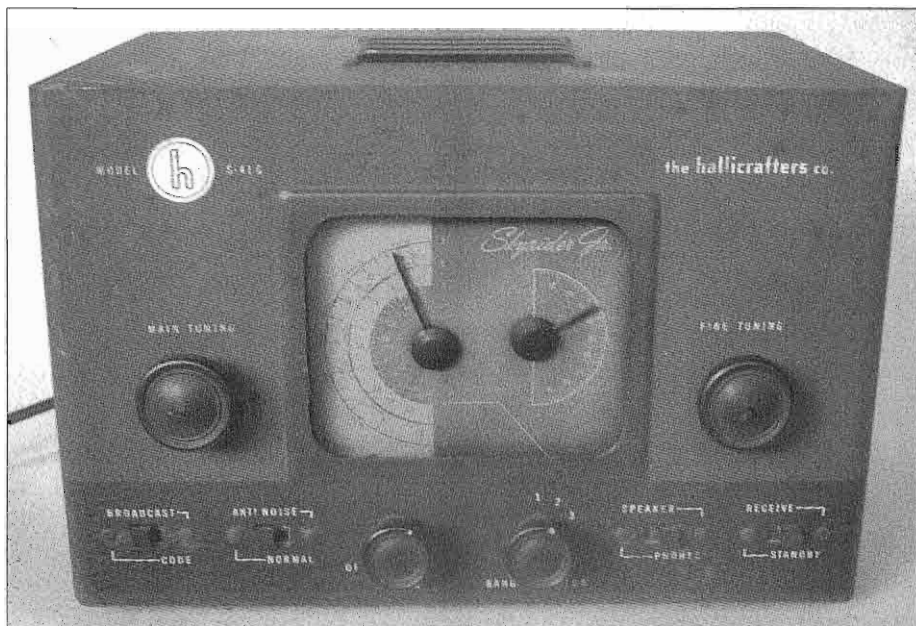
The early version of the S-41G "Skyrider Junior" has a bandspread dial that is calibrated from 0 to 100.
