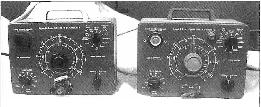
Pictured above are two versions of the popular and useful Heathkit C-3 Condenser Checker.
