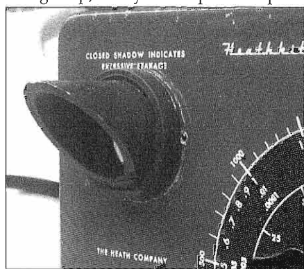
Figure 6: The homebrew eye shade is made from PCV pipe, as described in the text.
