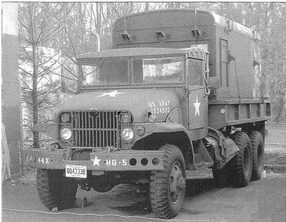
My 1952 GMC M211 2½-ton Army truck has been authentically restored to carry the AN/GRC-21A equipment shelter.
