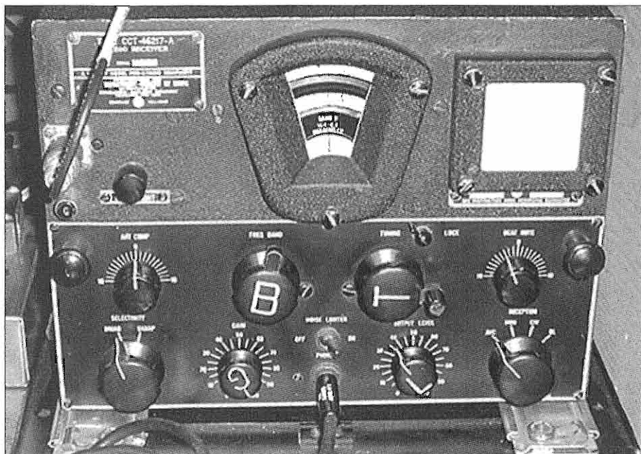
The RBM receiver with its mounting base attached and the new chart type.
