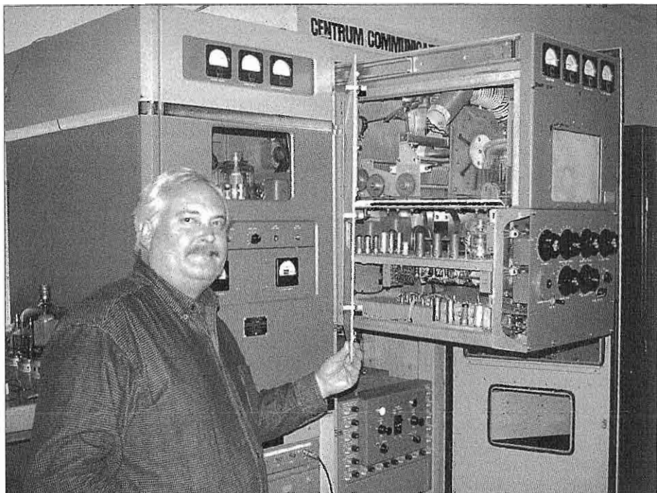
The author is shown with the AN/FRT-24 roll-out RF deck extended.
