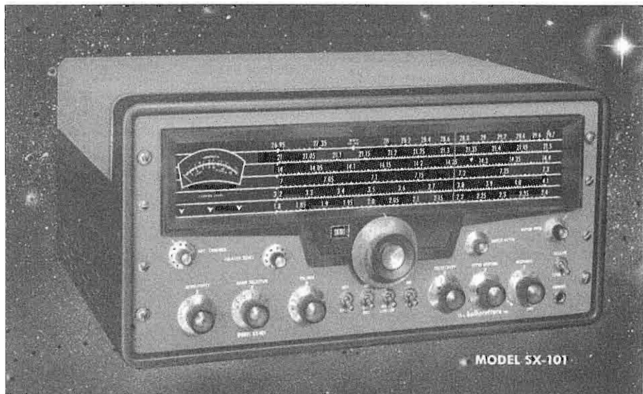
Above is a partial reproduction of Hallicrafters' ad in the catalog section of the 1957 ARRL Handbook. Notice the mechanical-digital band readout to the upper left of the main tuning knob.
