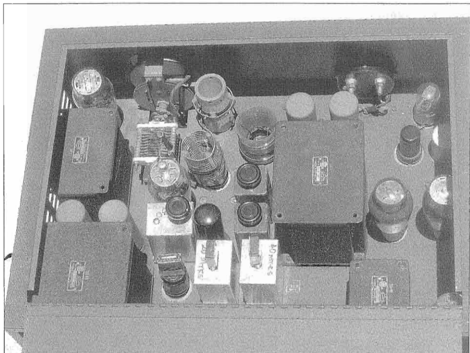
Figure 3: The inside topside. RF power supply is on the left, RF section in the center, and modulator and its power supply on the right.
