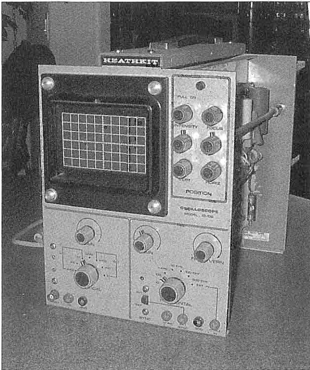
The Heathkit oscilloscope that I converted into an AM modulation monitor.
