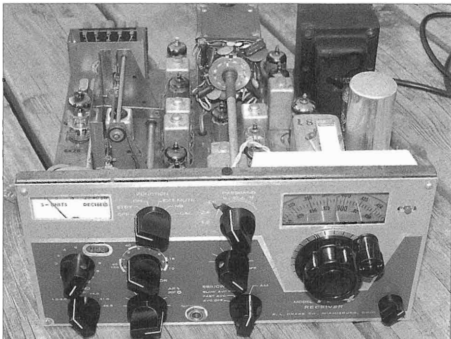
The Drake R-4 receiver with the cabinet removed. The knob on the lower left is the noise blanker threshold control.
