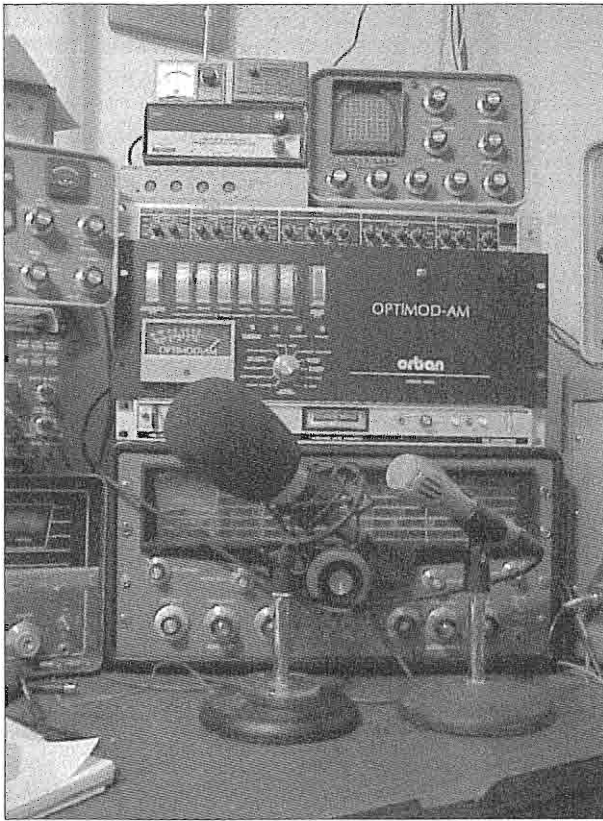
Figure 2: In front of the my SX-101 receiver is the “Hy-ball” (right) and B-1 (left) mikes. Between the receiver and an Optimod 9000A is the CBS Labs Volumax 4000. Sitting on top of the Ultra-Voice VX-2000 is the Aphex DA and Monitor scope. The little Behringer Shark is beside the field intensity meter.
