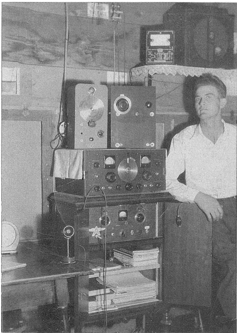
Above: Sylvan Smith (W7IFJ) at his station sometime after 1936. The two pieces of equipment on top of the Hallicrafters Super Skyrider are test equipment. Under the SX-17 is a homebrew transmitter built by W7IFJ. Sylvan is 91 and still active, but not on the air. (Photo courtesy Cliff Appel, W7CGA)
