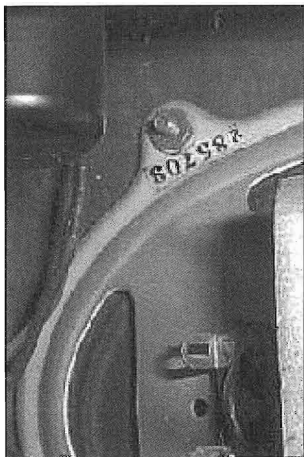
Figure 2: The speaker above carries the date cod of "285703." The number sequence "285" means the manufacturer was Rola, and "709" represents the 9th week of 1957.
