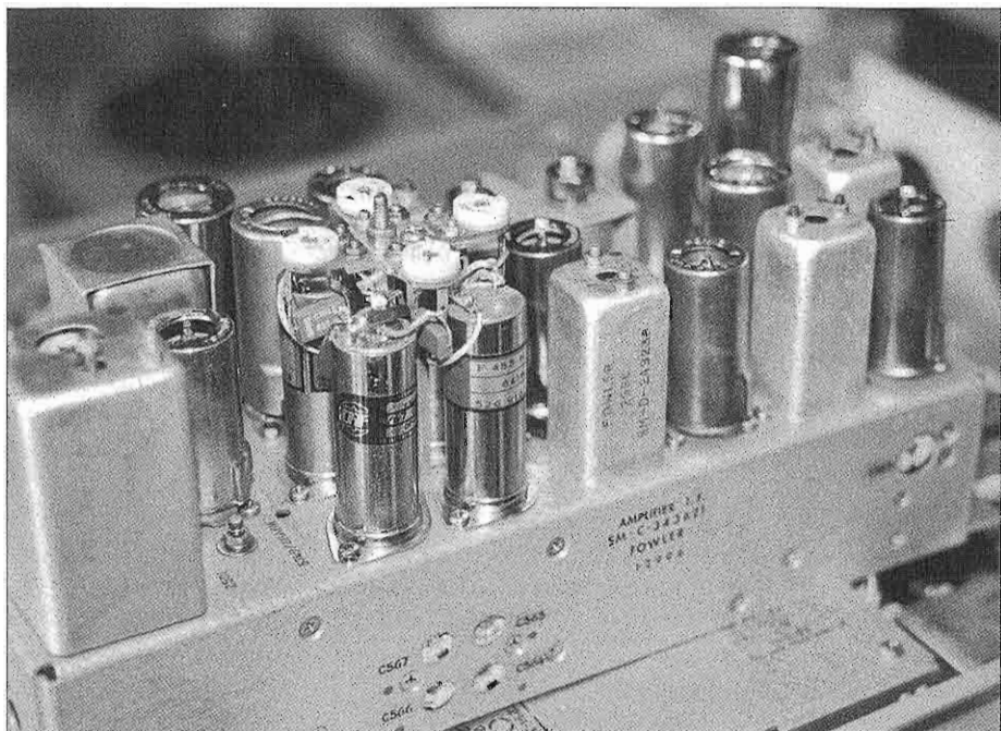
Figure 6: Left-side view of the IF subchassis with the filter cover removed that shows the D-F mechanical filter (foreground, left) and the Fowler markings, which have been silk screened on the chassis and stamped on an IF can.
