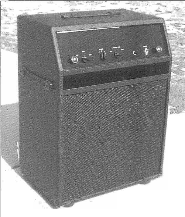
Figure 2: The outboard 15-inch speaker system has my amplifier mounted above the base reflex port as shown in this view.
