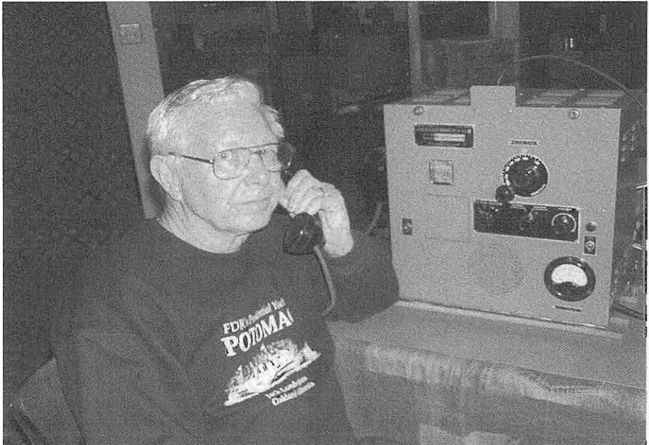
W6JRY is on the air with his restored 1942 BC-441D.
