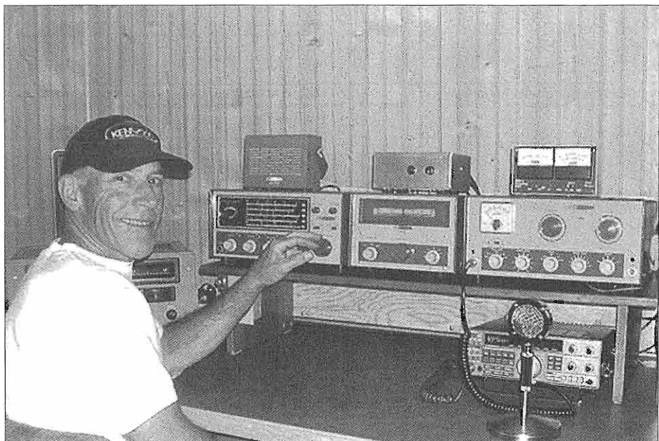
Above: Dick Geordan (W6SGJ/7) operates great vintage stations from Vancouver, WA. Here are 2 of Dick's AM stations, which are an Eico 720/730 combo and a Heath DX-60A/HG-10/HR-10 combo. The DX-60A and HG-10 his originals from the 1960's, and he restored and added the HR-10 about two years ago. More examples of Dick's equipment will be featured in an upcoming Photo column.
