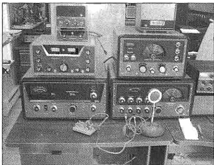
The Hallicrafters station consists of famous equipment such as an SX-117 and HT-33A (left) and the SX-115/HT-32 combo on the right.
