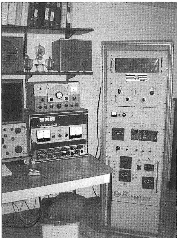
The completely rebuilt RCA transmitter at N2BC. It's now in a standard rack cabinet and modified to make it fully bandswitched from 160M through 10M. Notice the Ranger II driver and R-390A receiver. A good example of a quality transmitter that might be found for very little cost.
