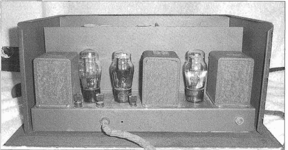
Rear view of the SW-5 with the covers removed.
