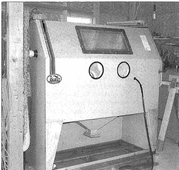
The installed bead blaster in my garage.
