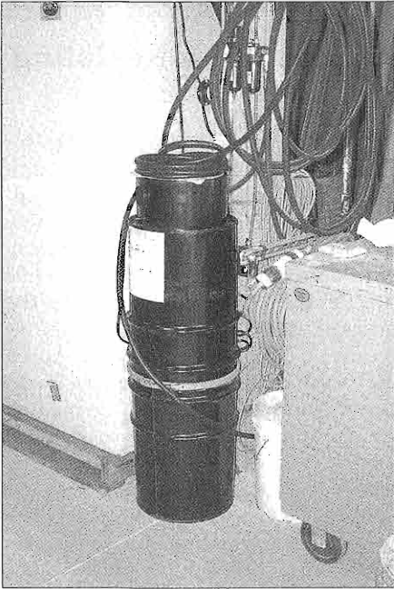
Here is the vacuum recovery system alongside the blaster cabinet.
