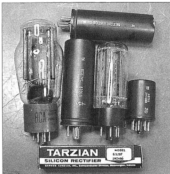
A collection of vacuum rectifiers and their solid-state replacements.
