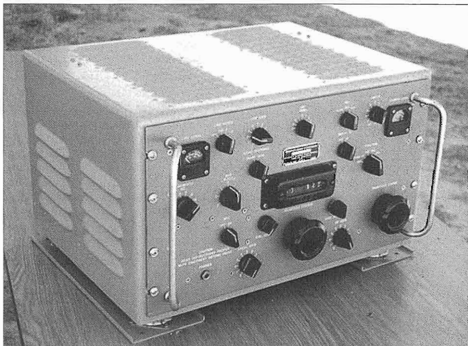
Figure 1: My Stewart Warner R-390A and its matching CV-979 tabletop cabinet.
