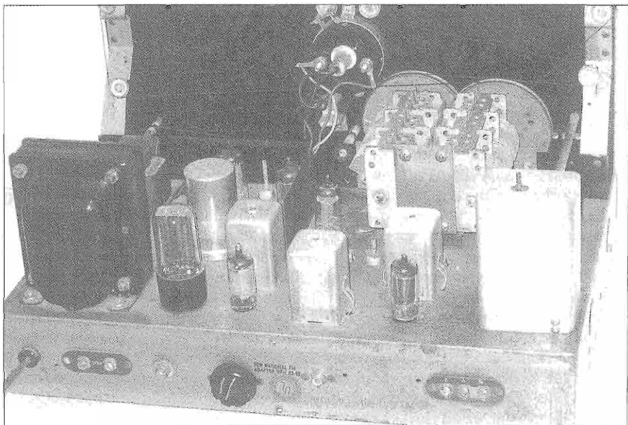
The rear of the NC-98 show the tube placement and the temperature-sensitive tuning condenser.
