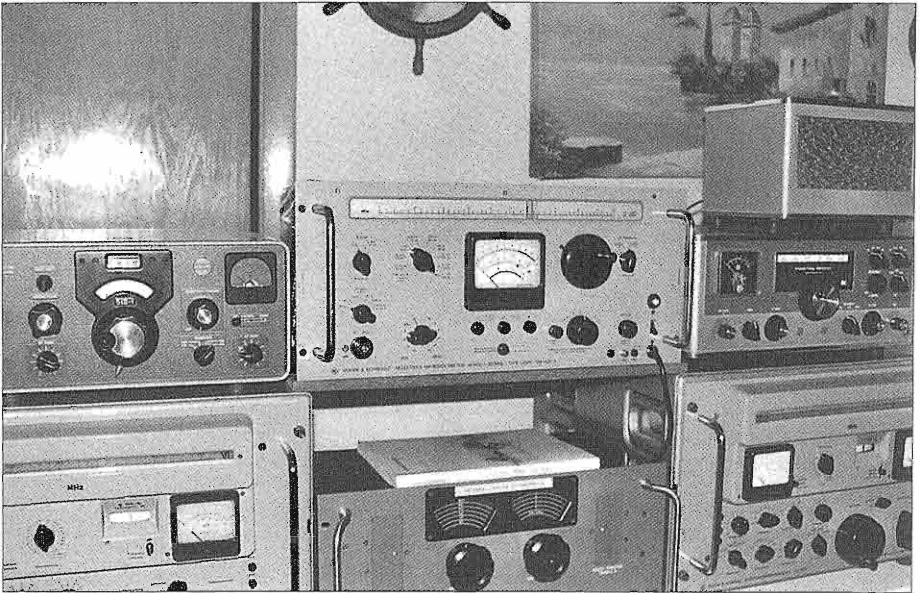
The author's receiving station showing the Rohde & Schwarz USVH frequency selective microvoltmeter in the top center, now in use as a sensitive receiver.
