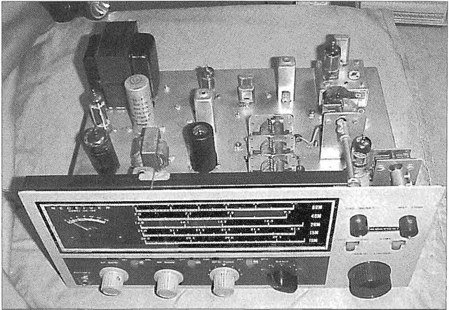
Top-front view of the author’s restored Heath HR-10B receiver. Designed as a 5-band, 7-tube, entry-level receiver that matched the DX-60 transmitter, it was available for 8 years, from 1967 to 1975.
