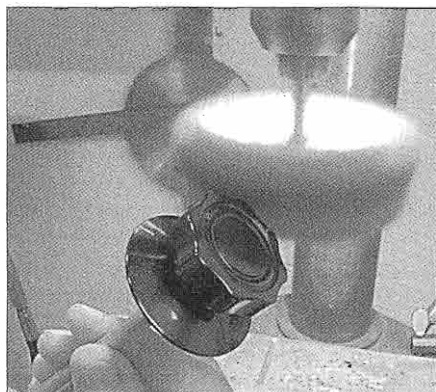
Polishing a knob using a small 6-inch buffing wheel in a drill press.
