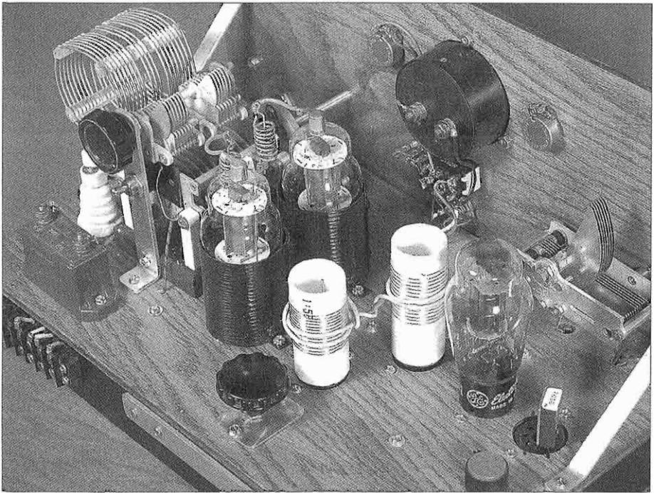
Here is a rear view of the RF deck on my recreated 1936 CW transmitter.
