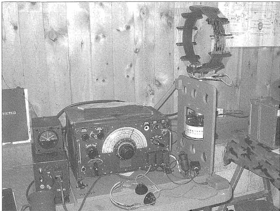
Lancaster bomber radio and a model of the Type 3 DF antenna. (KW1I image)
