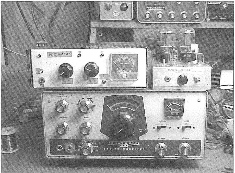
Figure 1: The HW-100-AM with two series-cathode modulators on top of the Heath transceiver. The one on the left has a plate meter to replace the lost plate metering function. The other is the prototype described I described in ER #191, April 2005.
