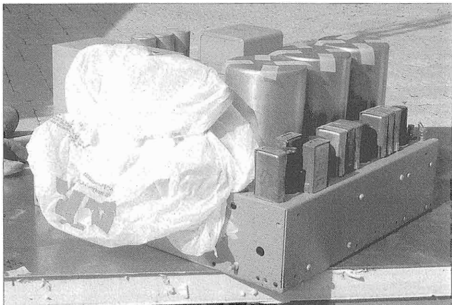
The main chassis is masked off and ready for the wash.
