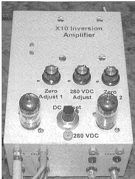
Figure 2: Vacuum tube amplifier with a gain factor of -10 and a DC offset up to 100 VDC. Box lettering is made with black printing on clear mailing labels.
