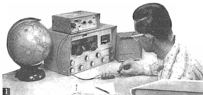
Novice transmitter shown here atop a Knight-Kit receiver, is powered by an external power supply, permitting fixed or mobile use. Inset shows closeup of transmitter face.
