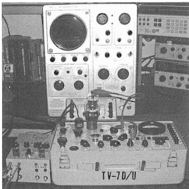
Figure 11. Test setup for characteristic measurements of a 1625 beam power pentode with a TV-7D tube tester and the times-ten DC amplifier connected to a Tektronix 575 curve tracer. The wire connections are given by Figure 1 of part 1, ER #212, page 24.
