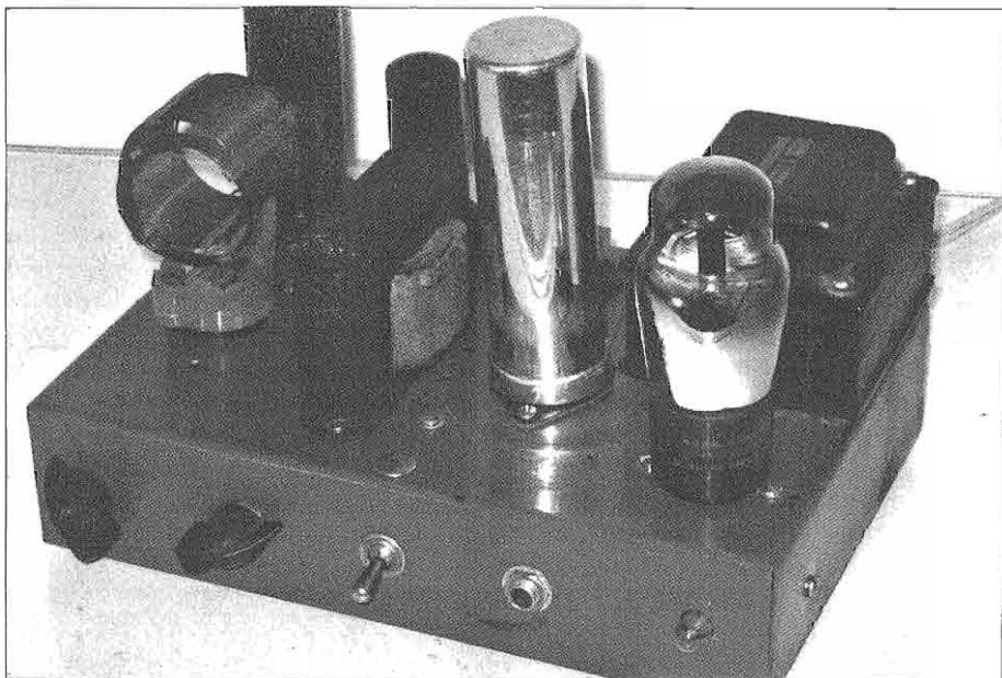
The Stancor 25B, has been rewired for 3 tubes, a 6AG7, 6L6, and a type 80 rectifier. It uses a Bud 80-meter coil on the left side of the chassis.
