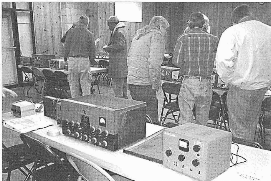
On the left, a Johnson Viking II is on display. To its right is a scarce Allied Knight transmitter, one of the 255 series, made from 1956 into 1961.
