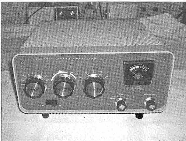
The Heathkit SB-200 amplifier that is the subject of this article (Photo by Bob Richmond, W8MNQ).
