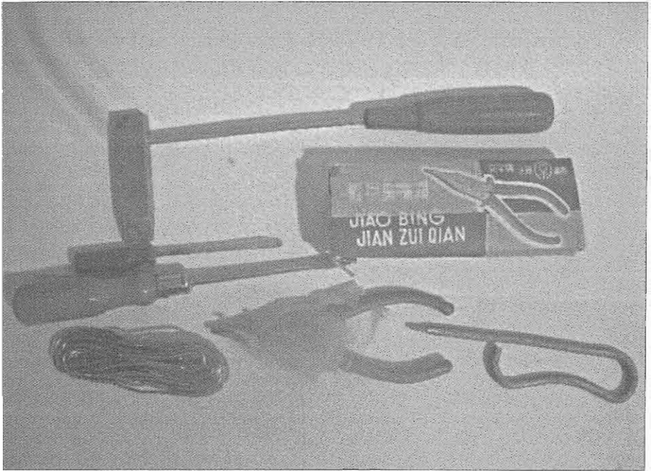
Figure 4: The Chinese Tool Kit Furnished with the GRC-9 Copy
