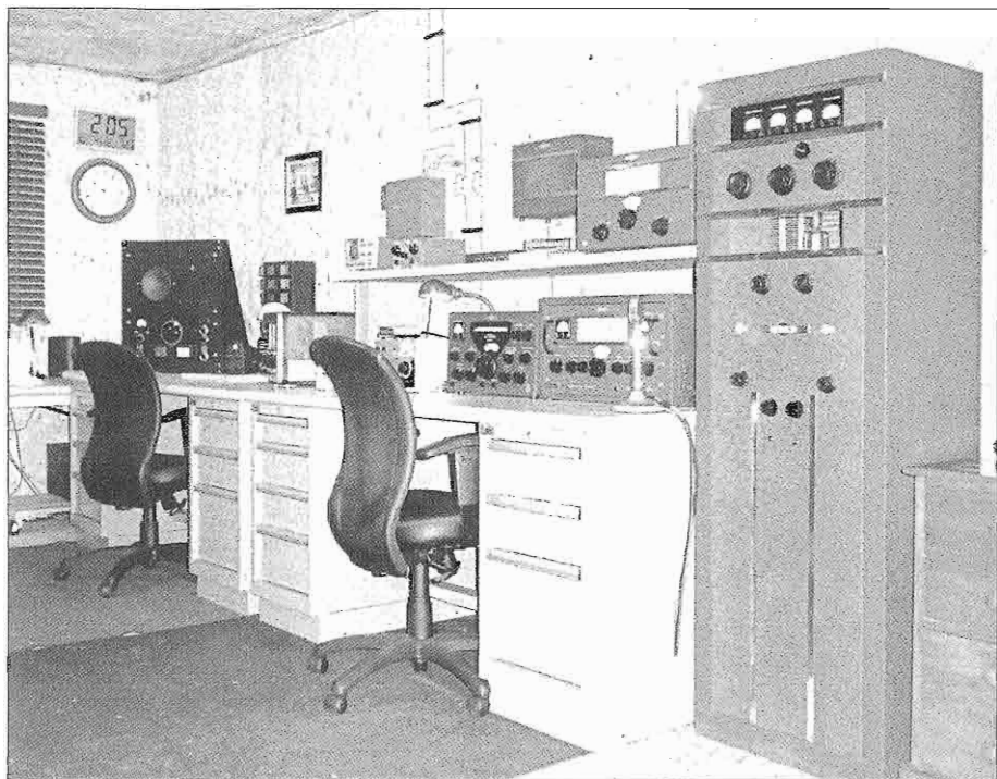
The Collins 30K-1 time capsule station of W7MGA is now in service at W1UJR.
