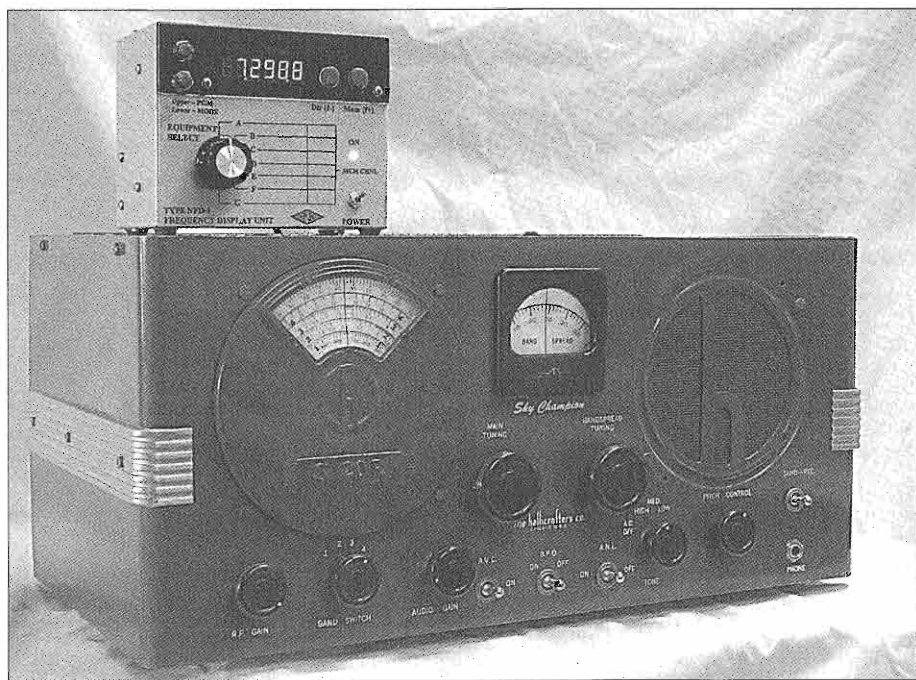
The National RF type NFD-1 digital frequency display is indicating where the Hallicrafters S-20R local oscillator is tuned.
