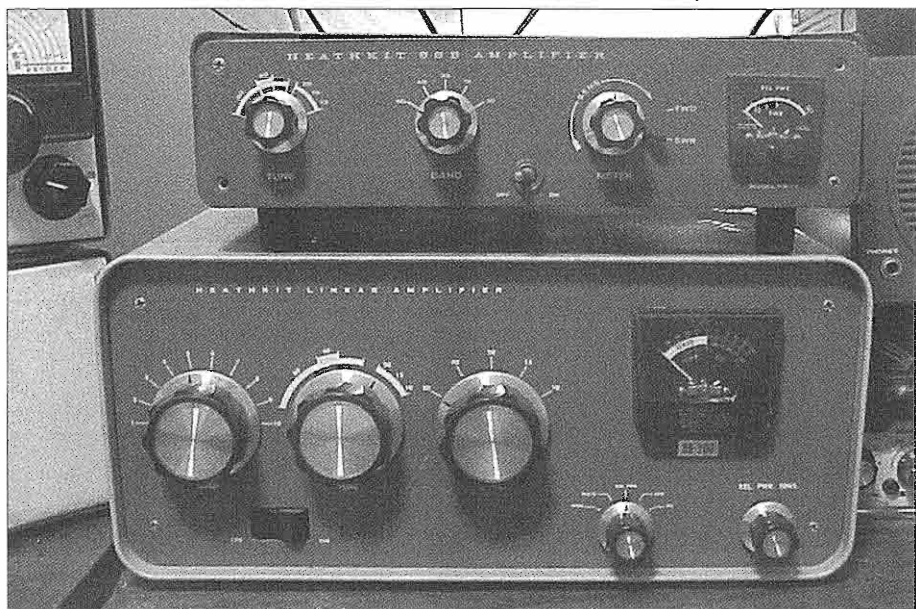
Pictured above are linear amplifiers, a Heath HA-14 "KW Compact" on top and the familiar SB-200 on the bottom.
