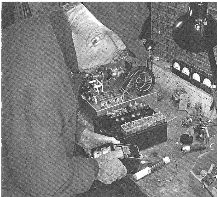
Checking the Plate Choke for Resonance with the Trusty Millen Grid Dipper
