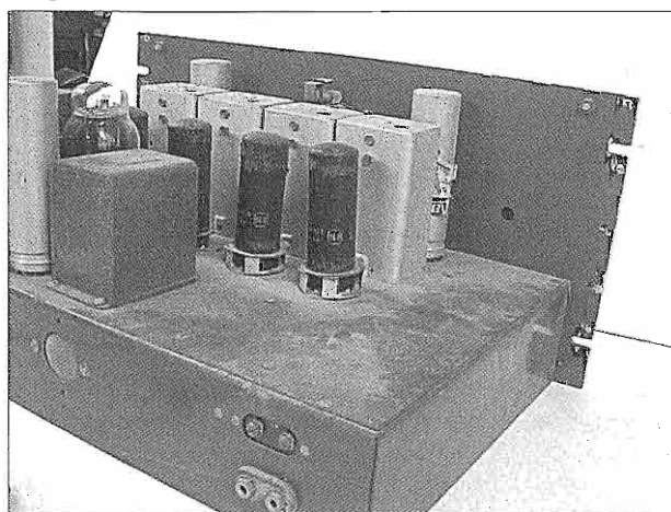
The rear view of the NTE-C shows a blank position where the audio amplifier has been omitted.
