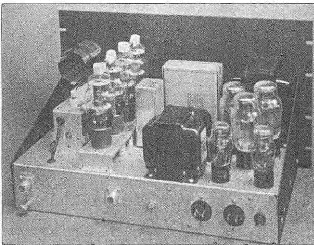
George Grammer's amplifier from April 1954, QST, using four 1625As in Class AB1, push-pull parallel.
