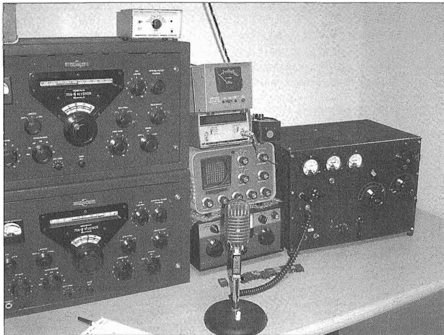
The author's AM station has the homebrew ART-14 transmitter on the right, and Collins 75A-2 and 75A-3 receivers on the left.
