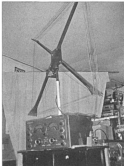
Figure 1: The 160-meter box-loop antenna is connected to the author's National NC-183D receiver.
