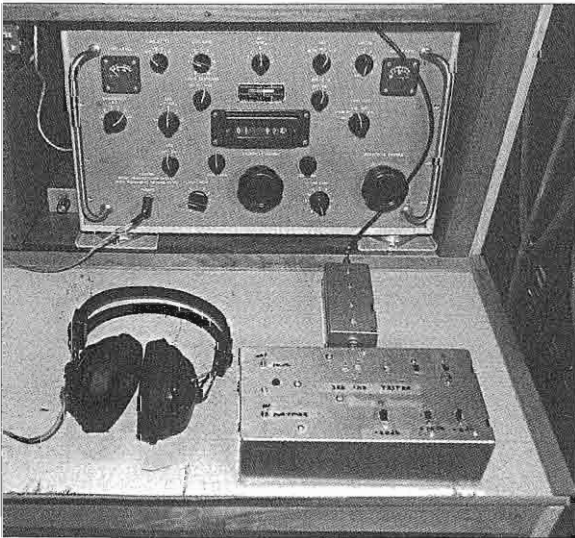
Figure 1: N6PY's IMD test box is shown connected to his R-390A/URR receiver.
