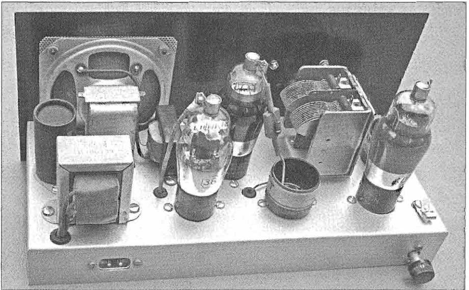
Rear view of reconstructed receiver showing original speaker, panel, RF and detector components with new one-piece chassis, audio tube, and power supply components
