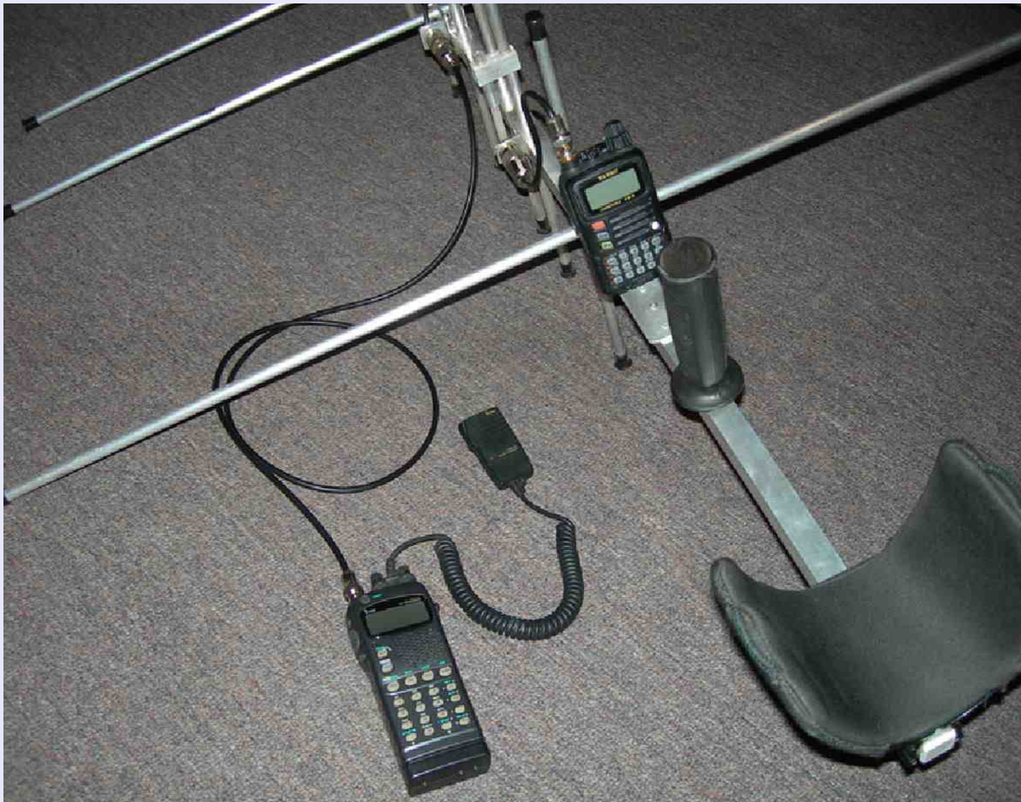
Yaesu VX-6R (70cm Rx) mounted on the boom, with Icom ICW-32E (2m Tx) that I clip onto my belt
