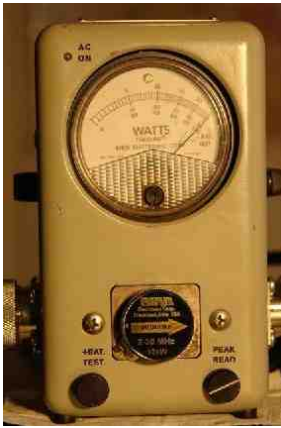
Fig.16: Proof of output power: With an input of only 70 W on 40 m the Tsunami power amplifier provides an output of 10.1 KW.
