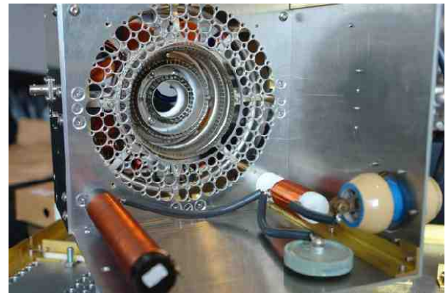
Fig. 7: RF insulation of the grid area from the plate area by a perforated metal plate of 4 mm thickness. The eight low inductive ground connection of the screen grid are visible directly behind the perforated plate. Instead of the smaller second RF plate choke a 2 pF capacitor was later installed for neutralization
