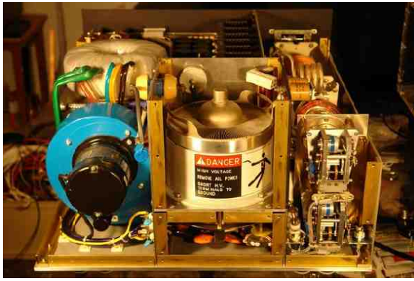
Fig. 10: Power amplifier without back board, the motors for the two vacuum
