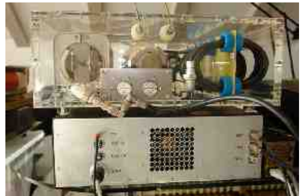
Fig. 17 – 19: The exclusive Tsunami capable antenna coupler in acrylic glass, working up to 15 KW SSB output in a frequency range from 160m up to 10 m. The integrated power meter (original Bird) exactly indicates forward and reflected transmission power, allowing for quick and accurate adjustment of the antenna. The coupler sits atop an amplifier with a 4CX1500B, which provides an output power of at least 2 KW SSB at a height of 16.5 cm.
