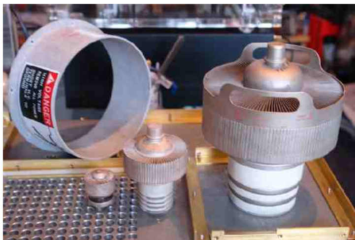
Fig.1: Size comparison: 4X150A, P_v = 250 W / 4CX1500B, P_v = 1500 W / 4CX10000D, P_v = 12000 W - The 322 holes in the 8 mm floor panel (underneath the transformer) are used as a cooling air intake.
