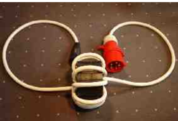
Fig. 20: Ferrite bead for 3 x 400 V power cord, weighing about 4 Kg.
