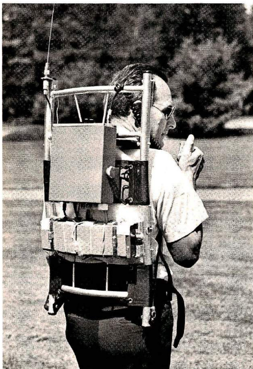
WA1QLI wearing the backpack portable two-meter transceiver, complete with batteries and antenna. The entire assembly weighs only 17 pounds and permits operation for up to 24 hours.
