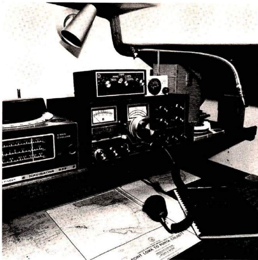
A neat shipboard Amateur radio installation using an older tube-type transceiver with a crystal-controlled fixed-frequency attachment. These rigs do their job well, but place a burden on the vessel's power source just to keep the tubes warm.
