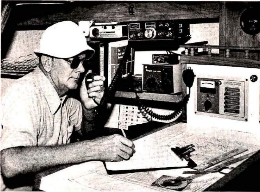
The author operating aboard his sloop Vector . This compact installation includes equipment for Amateur-band SSB, 2-meter fm, and vhf Marine Band operation. There is also room for an antenna tuner and a crystal-control adapter for the SSB transmitter.
