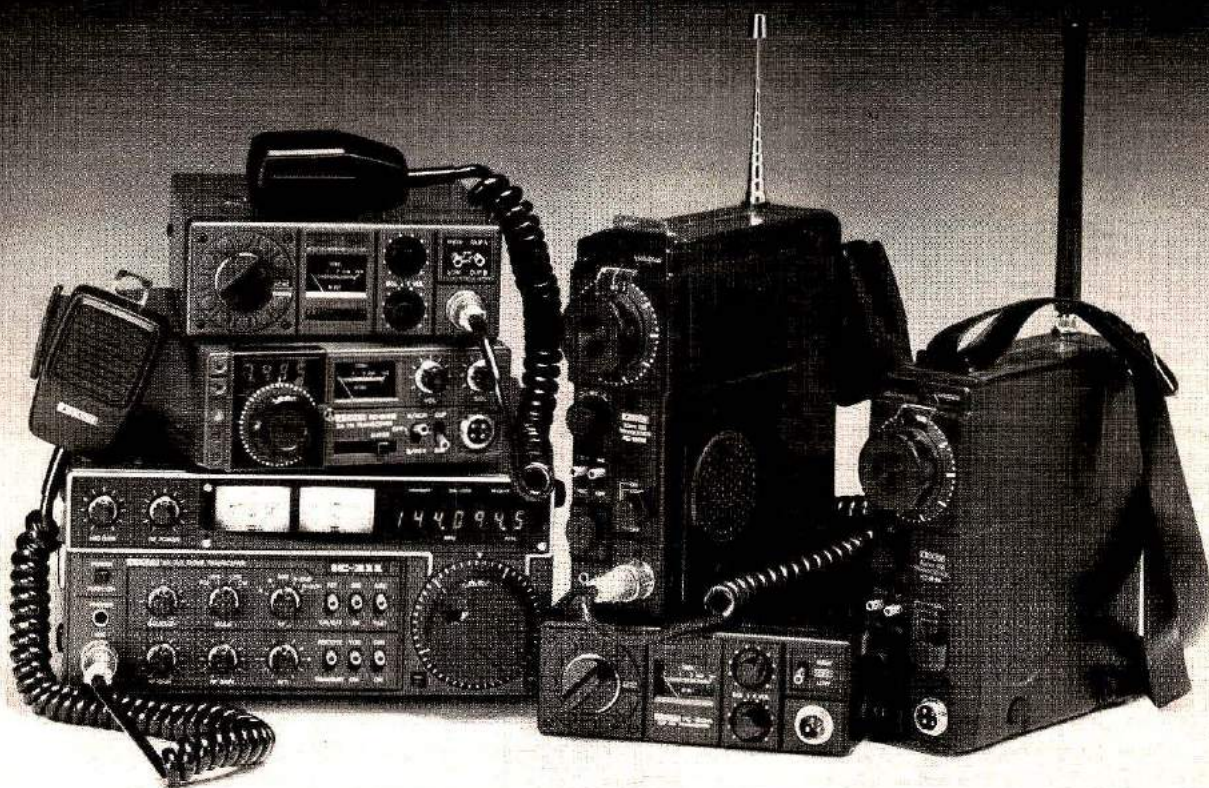
Clockwise from lower left: IC-211 4MHz, 2 meter, All Mode Transceiver; IC-245 Mobile 2 meter Transceiver; IC-22S Mobile VHF FM Transceiver; IC-502 Portable 50 MHz SSB Transceiver; IC-215 Portable 2 meter FM Transceiver; IC-30A Mobile UHF FM Transceiver.
