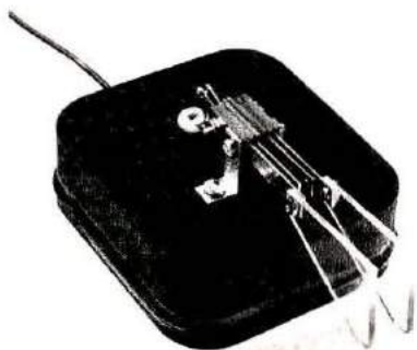
Fig. 1. My version of "El Cheepo" as it looks assembled. This version is set up as a "squeeze key," and the paddles are made of Plexiglas.
