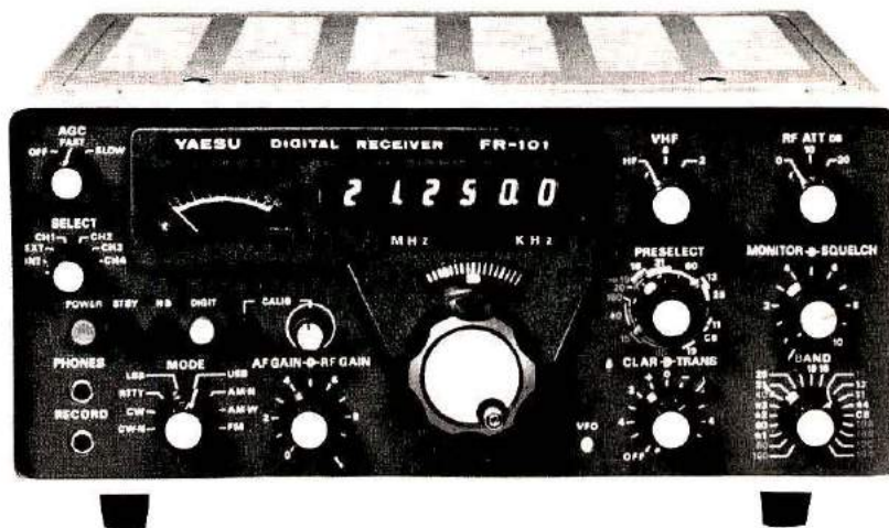
This Yaesu hf transceiver S-meter is calibrated to S9 plus 60 dB and therefore represents a total dynamic range of about 110 dB. Thus, the strongest signal that can be registered on the meter will be millions of times stronger than the weakest detectable signal. Actual S-meter readings will vary from band-to-band and from receiver-to-receiver. (Photo courtesy Yaesu Electronics.)
