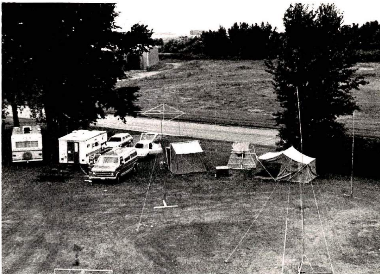
The station was set up in a park, and was housed in various tents, vans, and campers. Coverage was on 80 through 6 meters, and sometimes pileups were created when it became known that a North Dakota station was on! One neat trick for temporary mast support was the use of tripods mounted on 2 x 4 "T" frames.
