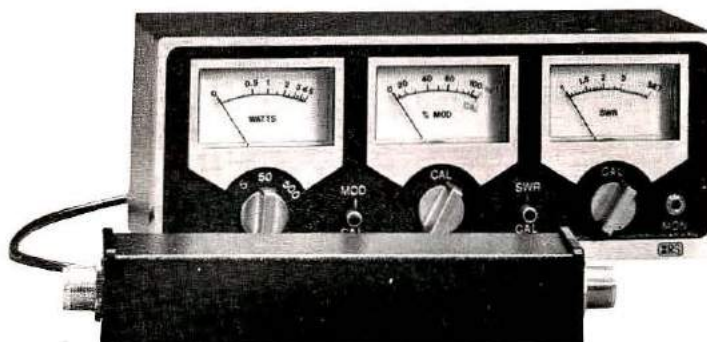
Besides measuring power and SWR, this meter will show the percentage of modulation of an a-m rig. In addition, the front panel monitor jack, with an earphone, lets the user listen to his signal.
