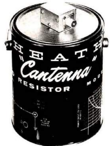
The Heath Cantenna is a valuable part of any shack. An oil-filled dummy load, it has a diode and meter jack to provide relative-power indications for tune-up purposes. Power rating is 1 kW.
