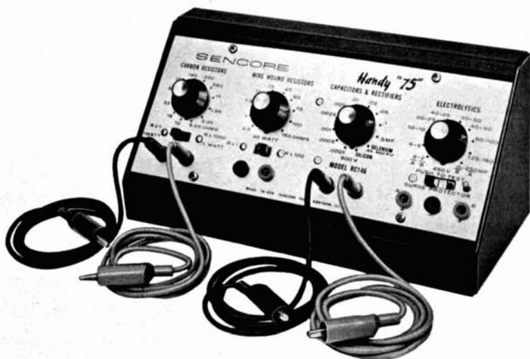
fig. 4. Commercially built parts substitutor saves carrying an inventory of small parts for test purposes.
